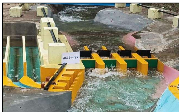
Simulation run for discharge of 4639 \text{ m}^3/\text{s}
