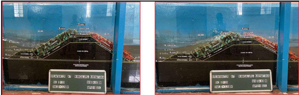
Wave action on armour layer of breakwater consisting of 7t tetrapod's at -3.0 m bed level with + 3.20 m water level and 4.80 m breaking wave height.
