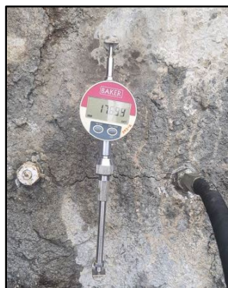
Vertical and horizontal test for determining In-situ Poisson's ratio
