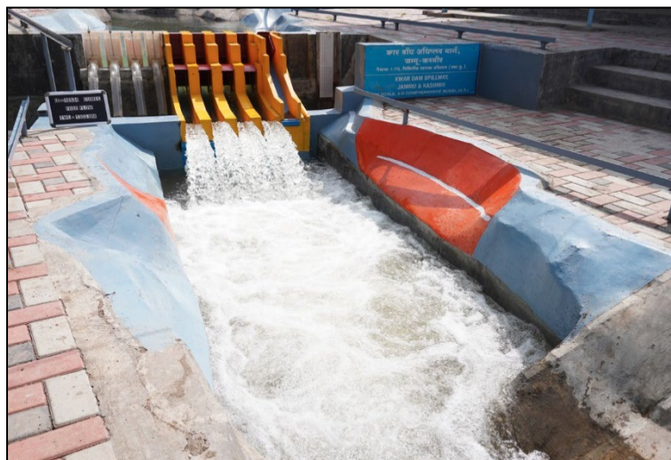
Flow Condition for Ungated Operation of Spillway for the Discharge of 10534 m 3 /s (100%) at RWL El. 1367.5 m
