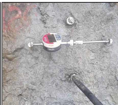
Vertical and horizontal test for determining In-situ Poisson's ratio
